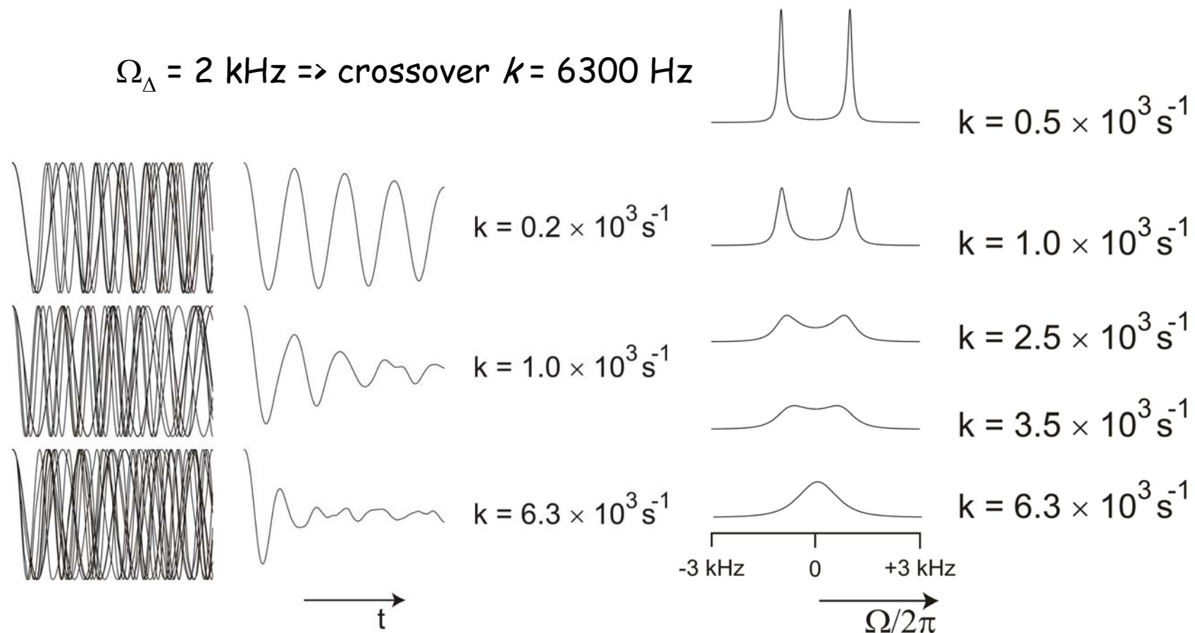
fast intermediate exchange:  $k > |\Omega_\Delta / 2|$
